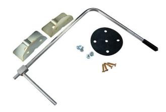
The AA18, AA19 and AA20 stainless steel pitot tubes are constructed from corrosion resistant stainless steel with permanently etched insertion depth graduations for a lifetime of service. The static pressure port is parallel to the sensing tube to allow quick, easy alignment of the tube with air flow. A universal model fits the user supplied 3/4" schedule 40 pipe in any length.
