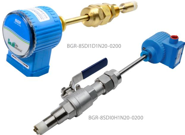
The direct insert style liquid flow sensor with stainless steel/PPS plastic or PEEK plastic tip combines flow sensing with a built-in transmitter for an all-in-one flow measuring system. This device fits all 1-1/2" to over 36" (38 to 915 mm) pipes, and it is intended for direct installation into the pipe through a 1" NPT hole.
